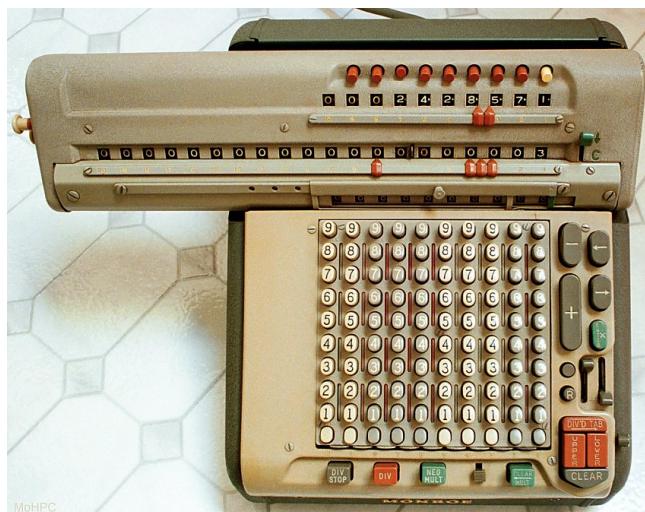
Figure 1: Monroe CSA-10 Mechanical Calculator using decimal arithmetic.
